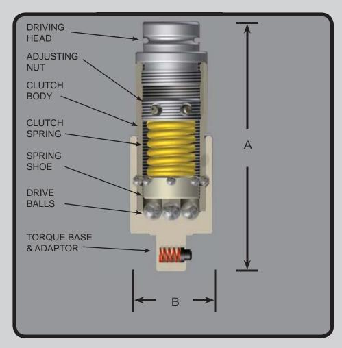
TITAN TORQUETTE® is a simple, reliable, and durable rolling element clutch with an improved design that reduces friction and improves concentricity which allows the TORQUETTE® to be used on fully automated assembly machines.
